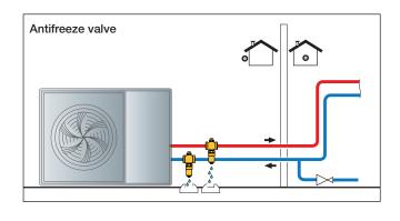
Leave at least 15 cm clearance from the ground (fig. A) to prevent the block of ice which may form below from stopping water from draining from the valve. Route the drain to a suitable collection point.
