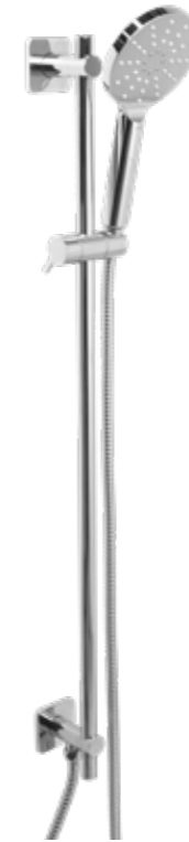
FWLO9516MCP with 3 spray functions Slide shower with integrated elbow, chrome, 900mm centres WELS 4 star 6.5L/min
