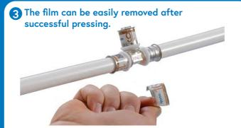
After pressing, a clear deformation of the stainless steel press sleeve is visible. In addition, the film can be easily removed after successful pressing (visual inspection).
