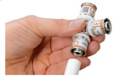
The pipe must be cut square at a 90° angle, insert the pipe into the fitting. The pipe end does not have to be deburred or calibrated beforehand.
