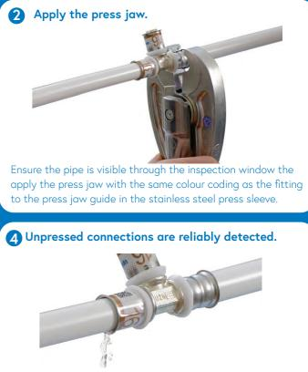
Unpressed connections are reliably detected as leaky during the leak test due to the unpressed-untight function. An unpressed fitting also stands out clearly due to the indicator foil still being present on the stainless steel press sleeve.
