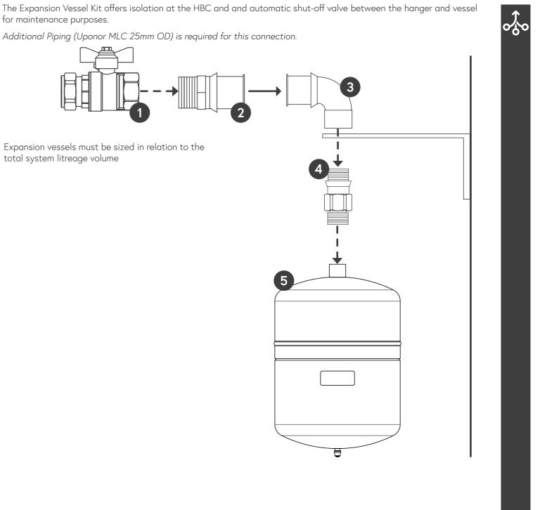
Expansion vessels must be sized in relation to the total system litreage volume
