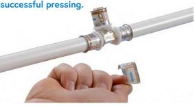
After pressing, a clear deformation of the stainless steel press sleeve is visible. In addition, the film can be easily removed after successful pressing (visual inspection).
