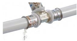
Unpressed connections are reliably detected as leaky during the leak test due to the unpressed-untight function. An unpressed fitting also stands out clearly due to the indicator foil still being present on the stainless steel press sleeve.
