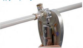
Ensure the pipe is visible through the inspection window the apply the press jaw with the same colour coding as the fitting to the press jaw guide in the stainless steel press sleeve.
