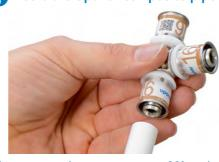
The pipe must be cut square at a 90° angle, insert the pipe into the fitting. The pipe end does not have to be deburred or calibrated beforehand.
